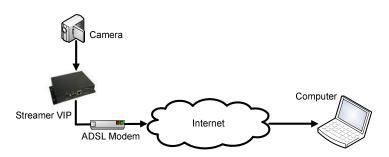
If your network accesses the Internet through a firewall or router, you can assign the Streamer VIP a private IP address. In this configuration, the IP address is not global. The following diagram illustrates the network topology for Private IP mode.
