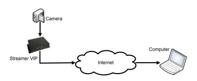
In the ADSL configuration, the Streamer VIP connects to the Internet using an ADSL modem. The following diagram illustrates the network topology for ADSL mode.
