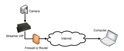
The Streamer VIP also supports networks that access the Internet through a relay server. In Relay mode, the Streamer VIP IP address is not global. The relay server must have one public IP address, and the relay server software must be installed. See Section 2.3.3 for information about the relay server software. The following diagram illustrates the network topology for Relay mode.
