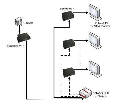
In a dynamic IP configuration, the DHCP server in the same LAN assigns the IP address to the Streamer VIP. The following diagram illustrates the network topology for dynamic local IP mode.
