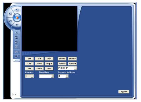
A Pan, Tilt, Zoom (PTZ) protocol defines camera control. Different camera manufacturers use different protocols, and there is no international standard protocol for all cameras. The Streamer VIP supports the PELCO-P/PELCO-D protocol defined by Pelco Inc.
