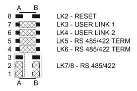
The following pages provide further information for each link. In each diagram the '+' sign indicates the default position for the link.
