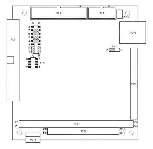
Below is a diagram showing the configuration of the links:
