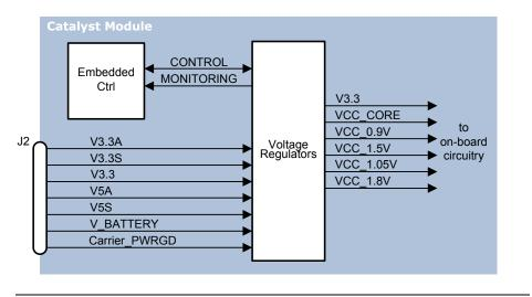
Note: The V5A rail should lead the V3.3A rail during ramp up or not lag by more than 0.7 V. The V5S rail should lead the V3.3S rail during ramp up or not lag by more than 0.7 V.
