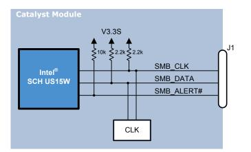
The following diagram illustrates the SMBus architecture on the Catalyst Module.
