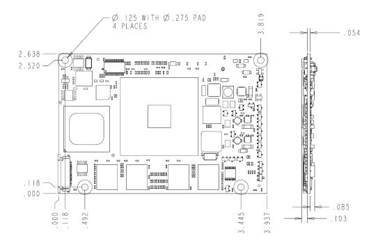
The next diagram illustrates the bottom and side views of the module. Notice connector J1 and J2 are located on the underside.
