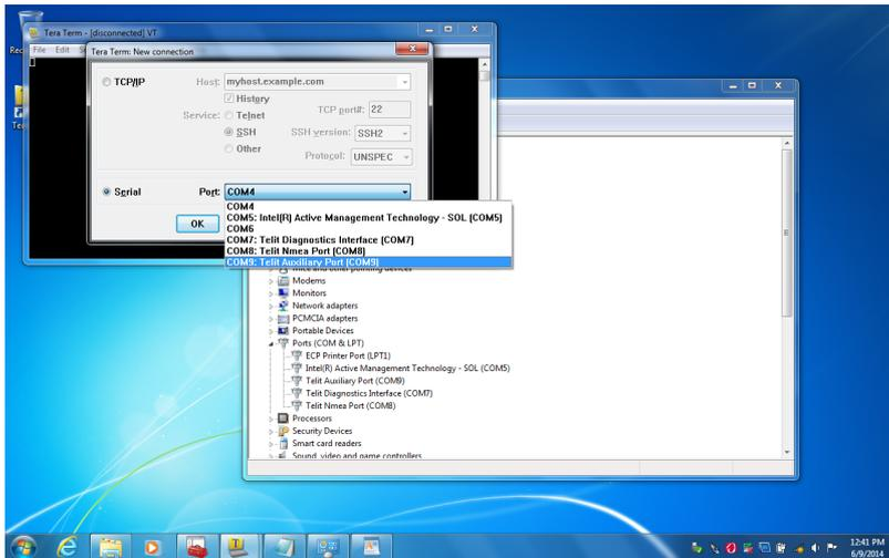
5. Once connected to the Auxiliary Port, provision the ReliaCELL 10-20-30 as follows:
